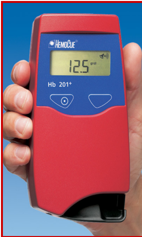
Figure 2 The HemoCue - a portable photometer.
