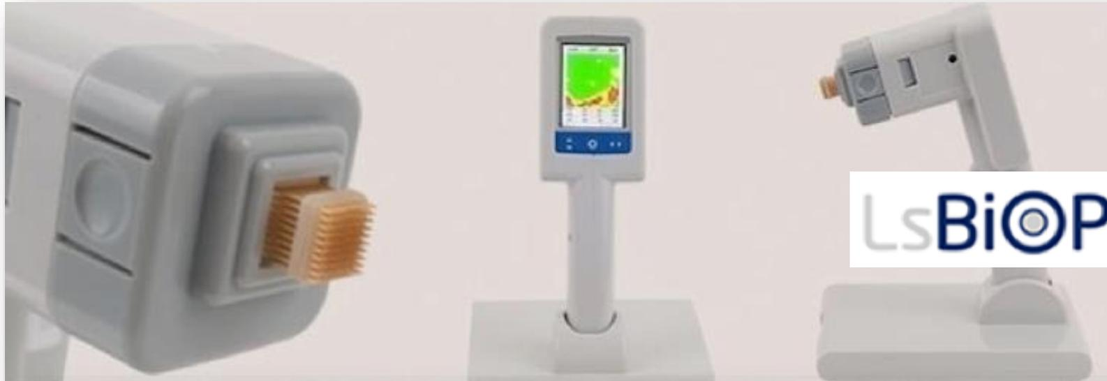
*TOUCH's* tissue imaging technology is based on clinically acceptable standards of bio-impedance spectroscopy. *TOUCH* provides real time images that depict the status of excised breast tissue margins. The device images an area of 13x13 mm with a spatial resolution of a fraction of a millimeter and penetration depth of several millimeters.
